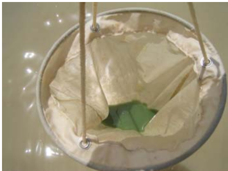
Figure 5: Sample (mesh size of the net: 20 \mu\text{m} ) collected in the Nombamba Reservoir (Mouhoun, April 2004, Céline Berger). Microcystin contents exceeded the recommended thresholds in this sample.
