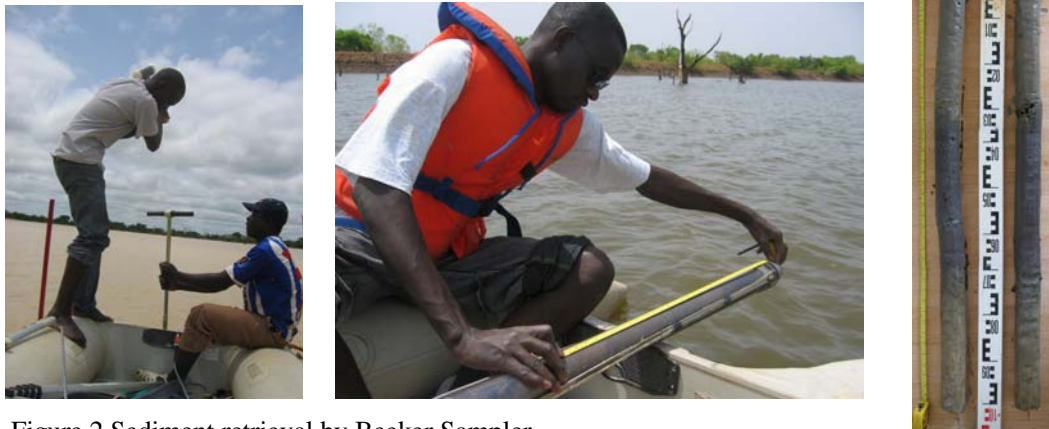
Figure 2 Sediment retrieval by Beeker Sampler
